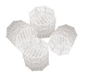
The high-capacity Octopac creates exciting new possibilities in packed tower design. The unique drip points and gas turbulence create millions of small droplets, multiplying the surface area for gas flow. The Octopac provides efficient heat or mass transfer with low pressure drop
